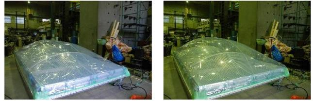
a. Initial shape at  $0 kPa$  b. Final shape at  $2 kPa$
