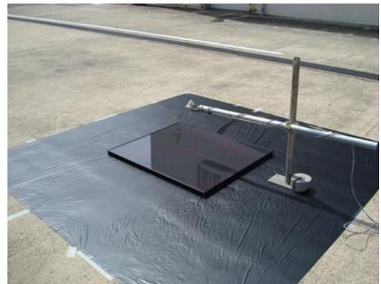
Fig. 11 Measurement for insolation reflectance of solar panels
