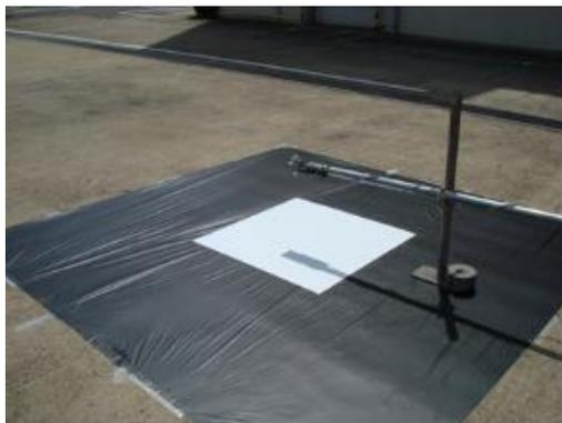
Fig. 4 Measurement for insolation reflectance
