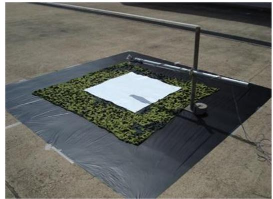
Fig. 10 Measurement for insolation reflectance of decorative nets
