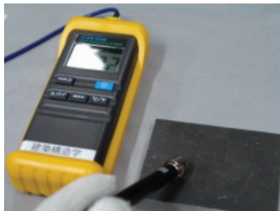
(b) Digital thermometer
